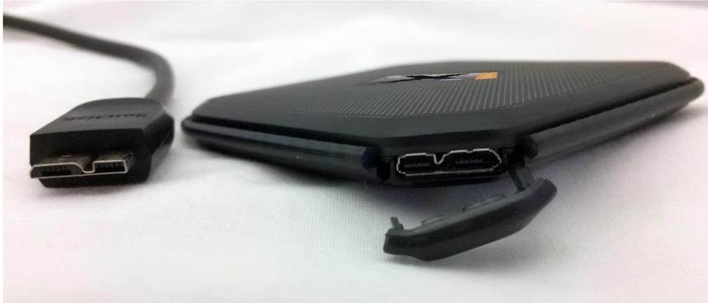
**Figure 280: Plug this end of the USB cable on the left into the SSD drive's input port.**
