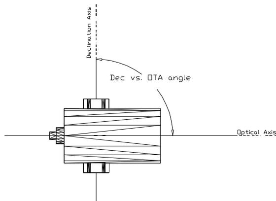
**Figure 34: Top view of a fork mount.**
