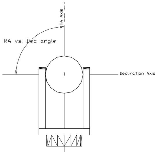
**Figure 36: The front view of a fork mount.**
