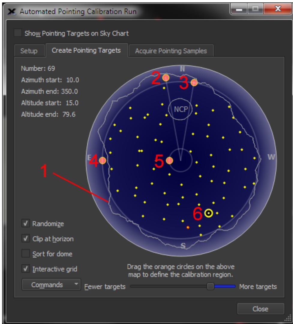
Figure 24: The *Create Pointing Targets* tab.
