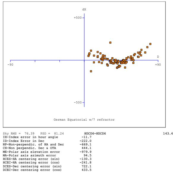
Figure 51: Before Adding the HXCD2 Term (RMS = 76 arcseconds).
