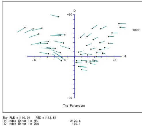
**Figure 43: Error vectors on a Cartesian Cylindrical projection.**
