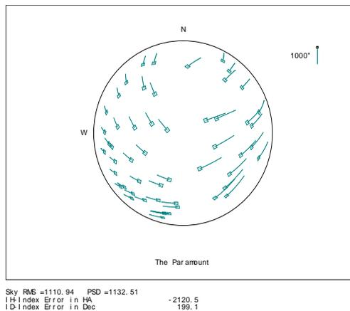
**Figure 42: Error vectors graphed using an orthographic projection.**
