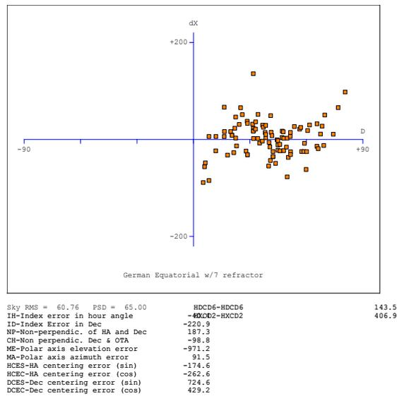
Figure 52: After Adding the HXCD2 Term (RMS = 61 arcseconds).
