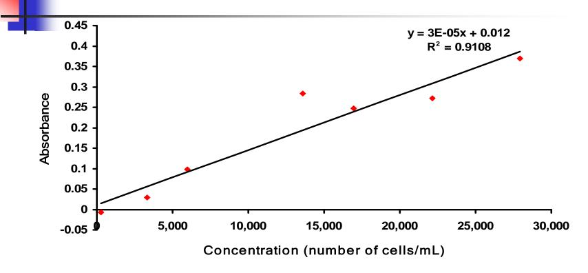
As cell concentration increases, the absorbance, which is directly proportional to amount of reduced MTT product, also increases due to the greater number of live cells which are metabolizing (n = 7)
