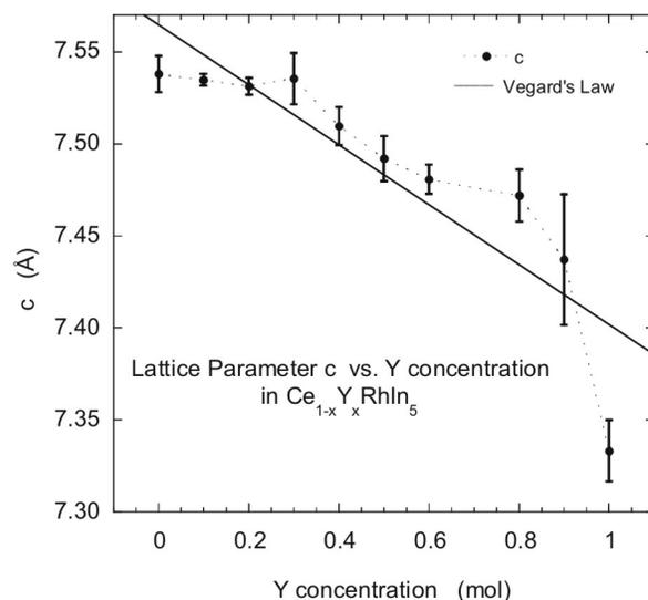
Figure 4. Tetragonal lattice constant  $c$  as a function of Y concentration  $x$  for the  $Ce_{1-x}Y_xRhIn_5$  system. The dotted line is a fit to the data and the solid line represents the linear relationship of Vegard's law.
