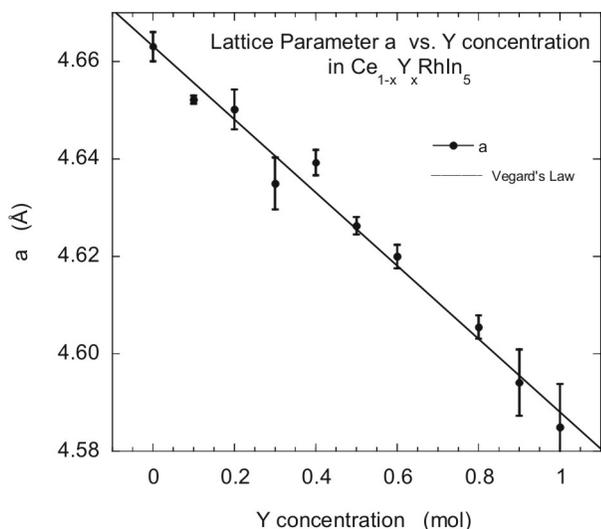
Figure 3. Tetragonal lattice constant  $a$  as a function of Y concentration  $x$  for the  $Ce_{1-x}Y_xRhIn_5$  system. The dotted line is a fit to the data and the solid line represents the linear relationship of Vegard's law.
