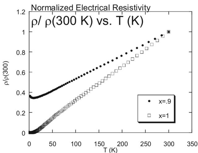
Figure 6. Electrical resistivity  $\rho$  normalized to its value at 300 K,  $\rho/\rho(300\text{ K})$ , as a function of temperature for  $\text{Ce}_{1-x}\text{Y}_x\text{RhIn}_5$  with  $x = 0.9$  and  $x = 1.0$ .
