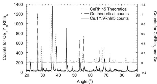
Figure 1. Graphical representation of the x-ray diffraction measurements for  $Ce_{1-x}Y_xRhIn_5$  against  $CeRhIn_5$  theoretical and Germanium theoretical. The graph is plotted as intensity vs. theta for  $20^\circ \leq \theta \leq 90^\circ$ .
