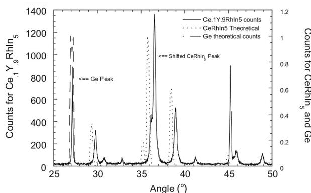
Figure 2. Magnified version of the graphical representation of the x-ray diffraction measurements for  $Ce_{1-x}Y_xRhIn_5$  against  $CeRhIn_5$  theoretical and Germanium theoretical. The graph is plotted as intensity vs. theta for  $20^\circ \leq \theta \leq 50^\circ$ .
