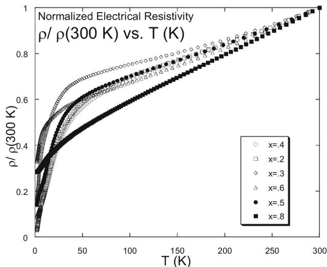
Figure 5. Electrical resistivity  $\rho$  normalized to its value at 300 K,  $\rho/\rho(300\text{ K})$ , as a function of temperature for  $\text{Ce}_{1-x}\text{Y}_x\text{RhIn}_5$  with  $0.2 \leq x \leq 0.8$  and  $x = 0.8$ .
