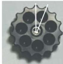
Figure 27: Each high spot or “tic” on the azimuth adjustment knob represents two arcminutes azimuth adjustment. The azimuth adjustment knobs are calibrated. One rotation results in 30 arcminutes of azimuth adjustment. Therefore, each “knob-tic” (that is, each high point on the knob itself, see Figure 27) equals two arcminutes.
