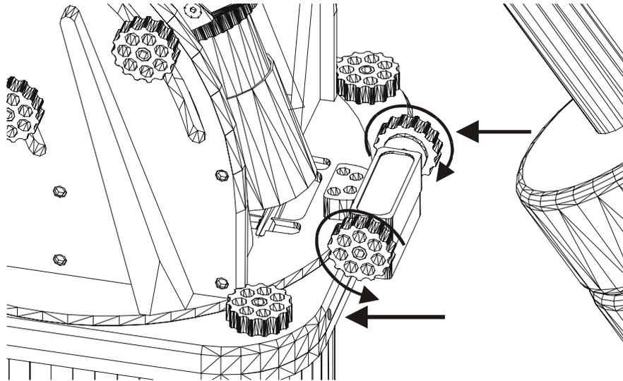
Figure 26: Azimuth adjustment knobs and tensioning screws.
