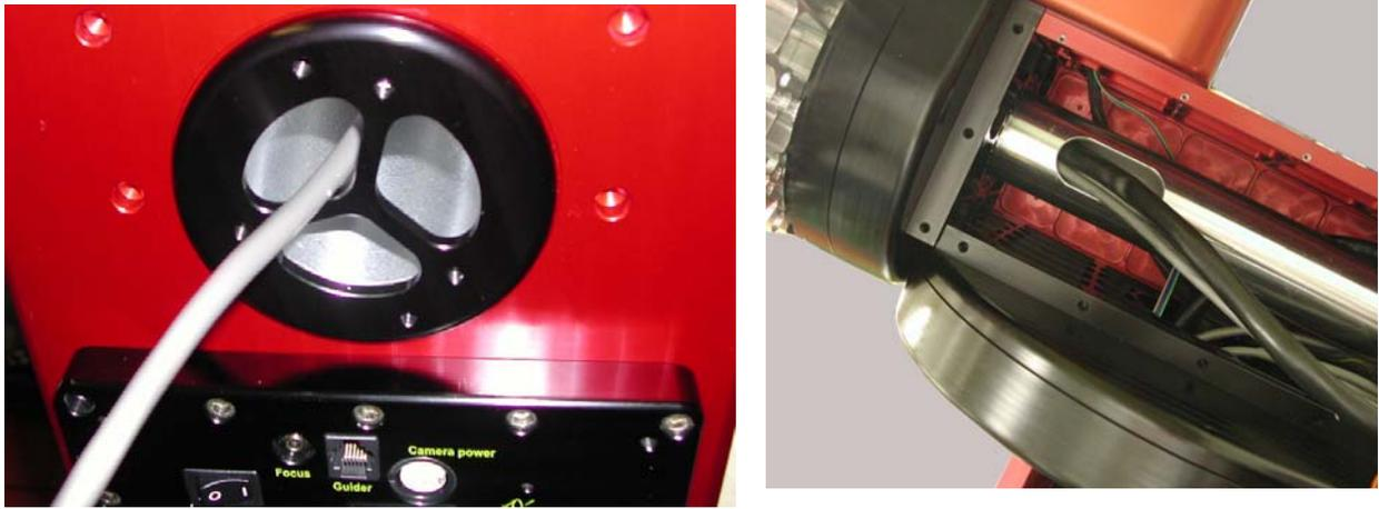
Figure 34: Route of “through the mount” cabling.
