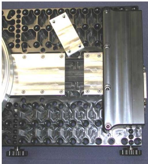
Figure 13: Channel Covers (unanodized for illustration purposes)
