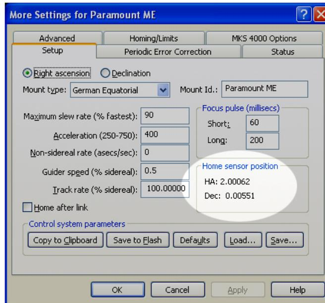
Figure 52: The homing sensor positions computed by TheSky6.
