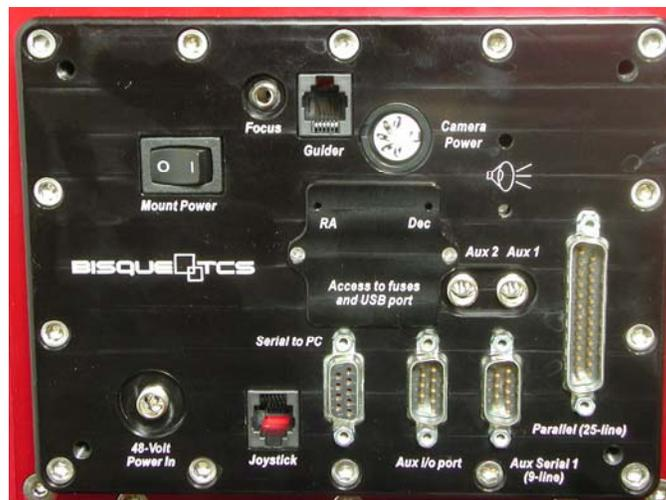
Figure 77: Use a small Phillips screwdriver to remove the cover labeled “Access to Fuses and USB Port” to access the USB port.
