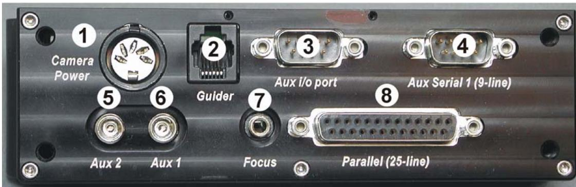
Figure 5: Instrument Panel.
