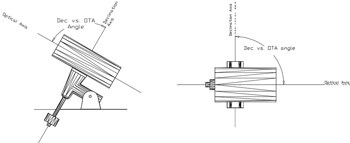
Figure 30: Try to minimize OTA non-perpendicularity errors.
