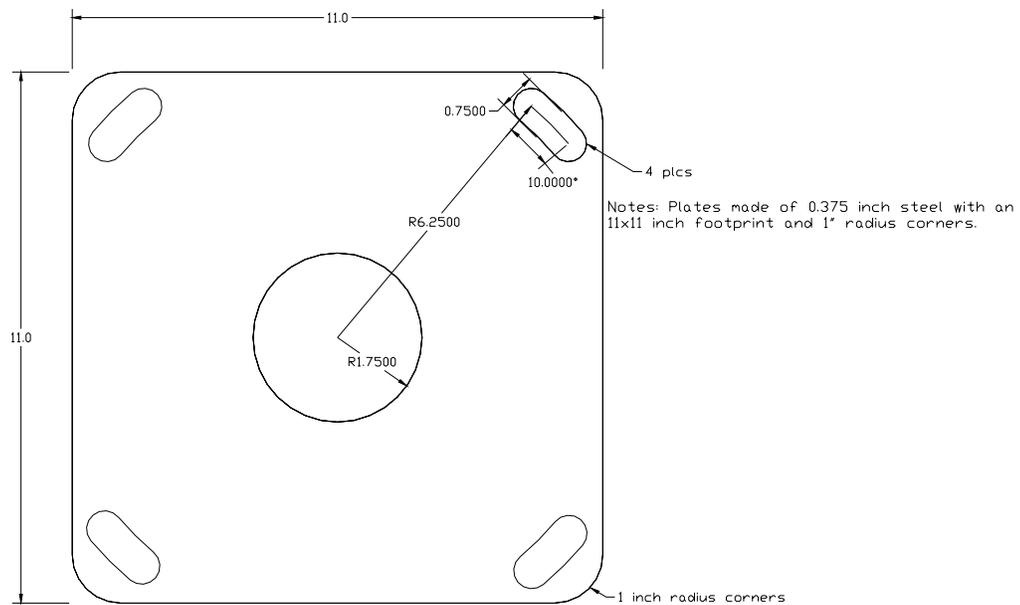
Figure 69: Dimensions of pier base plate.
