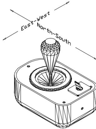
Figure 18: Slewing the Paramount ME with the joystick.
