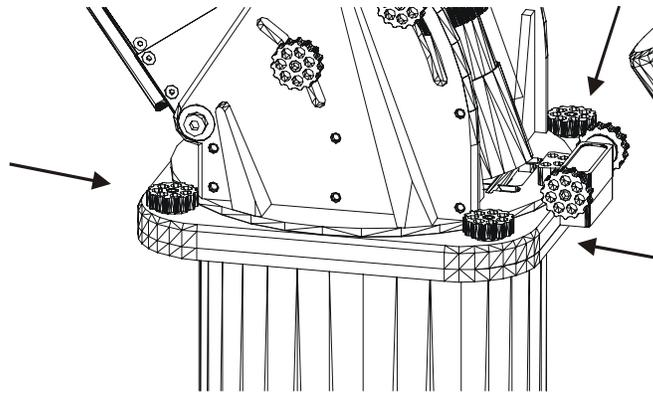
Figure 17: Location of Base Plate Attachment Knobs.
