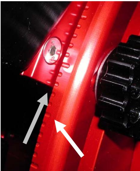
Figure 6: Wedge assembly altitude scale.
