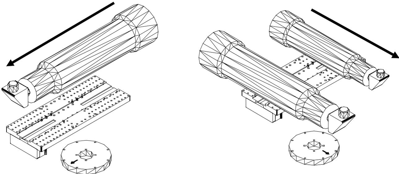
Figure 12: Typical (left) and wide (right) Versa-Plate mounting configurations. The black arrows indicate the direction of incoming light. Note that the machined arrow on the declination hub points *in the same direction* as the incoming light.
