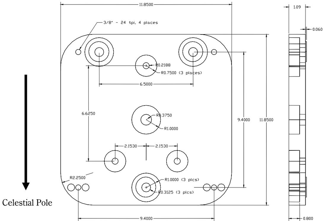
Figure 64: Base Plate dimensions (plan and side view).
