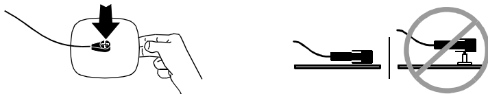
Figure 5-4 Connecting FAST-PATCH Electrodes to Defibrillation Cable
