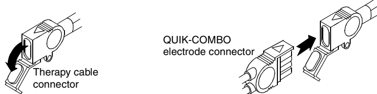
Figure 5-3 Connecting QUIK-COMBO Electrodes to Therapy Cable
