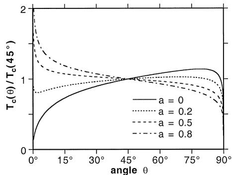
Fig. 1. Normalised crossover temperature  $T_c$  as given by Eq. (1), and for several values of the ratio  $a = H_{\perp}/H_{\parallel}$ .
