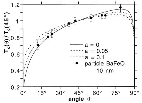
Fig. 2. Angular dependence of the crossover temperature  $T_c$  for BaFeCoTiO particle. The lines are given by Eq. (1) for different values of the ratio  $a = H_{\perp}/H_{\parallel}$ . The experimental data are normalised by  $T_c(45^\circ) = 0.31$  K.
