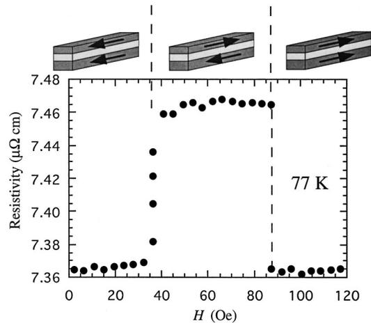
FIG. 3. Resistance as a function of the external magnetic field at 77 K determined by a four-point dc technique. The magnetic domain structures inferred from the resistance measurement are schematically shown.
