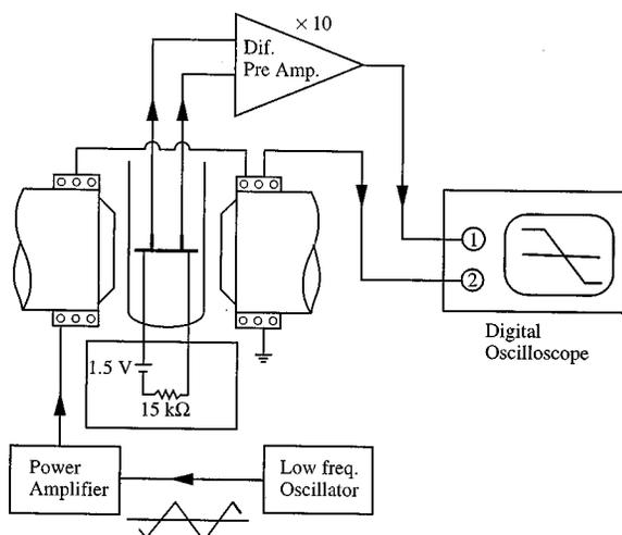
FIG. 2. Block diagram for the time variation measurements of the resistance during the magnetization reversal.
