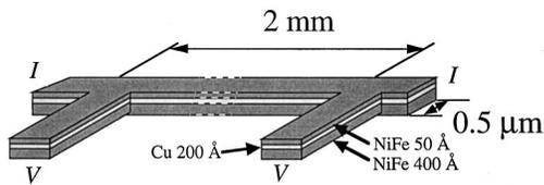
FIG. 1. Schematic illustration of sample structure. The width of the wire is  $0.5 \mu\text{m}$  and the sample has four current–voltage terminals where the voltage is probed over a distance of 2 mm.
