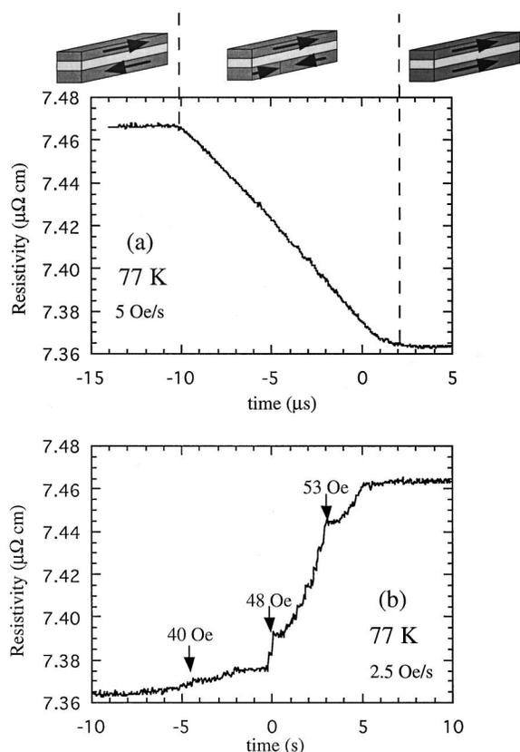
FIG. 4. Time variation of the resistance during the magnetization reversal of the (a) 400-Å-thick NiFe layer and (b) 50-Å-thick NiFe layer at 77 K.
