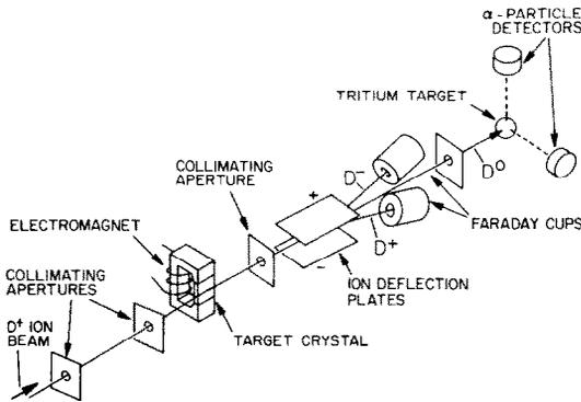
Fig. 1. Schematic diagram of the apparatus used in ECS experiments.
