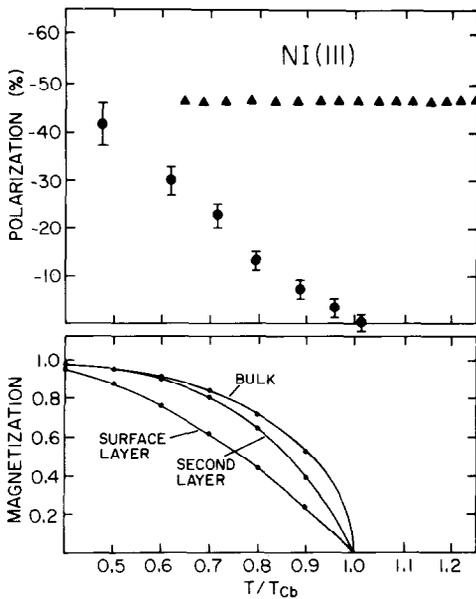
Fig. 2. Upper part:  $T$ -dependence of the long-range ESP (●) and of the “local” ESP (▲) at Ni(111) surfaces. Lower part:  $T$ -dependence of the first and second layer and the bulk in mean field theory [8].
