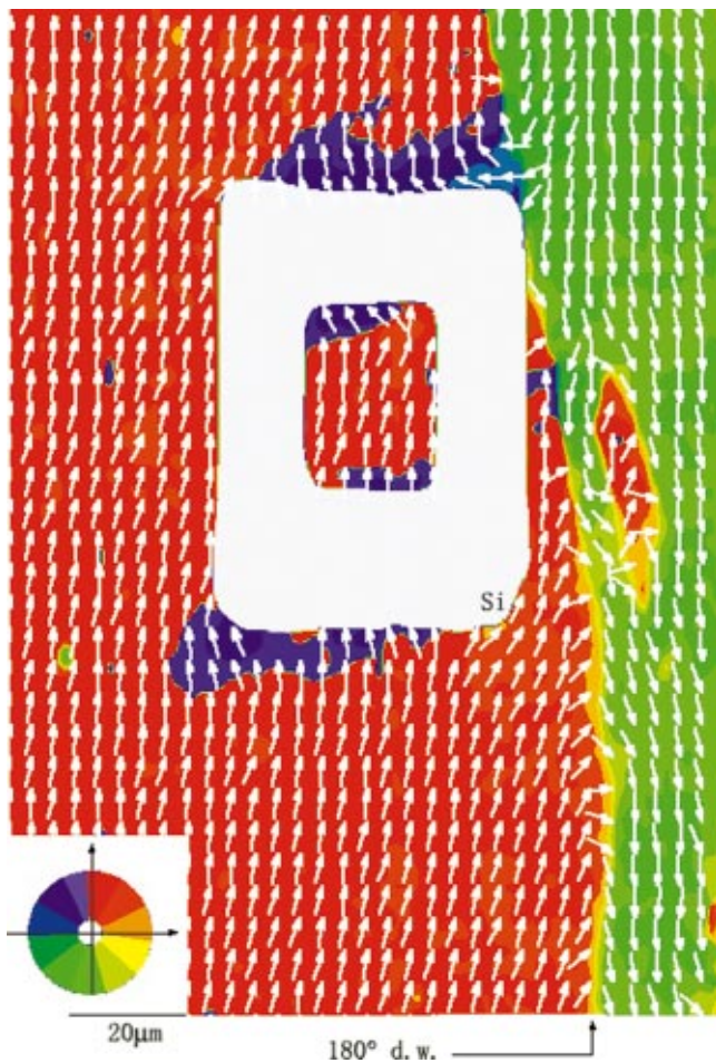
FIG. 1. Magnetic domain image (size: 200\ \mu\text{m} \times 140\ \mu\text{m} ) of the surface of a 30 nm thick Co/Si(100) film with a magnetic element of size 30\ \mu\text{m} \times 21\ \mu\text{m} created by ion beam milling and color wheel in the lower left part of the figure.
