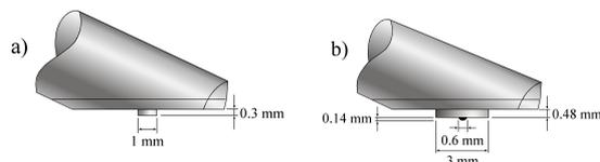
**Figure 1.** Schematic presentation of the original (a) and novel (b) indentation instruments.
