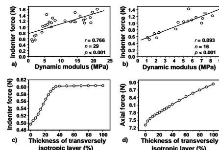
**Figure 3.** Experimental correlations between the instantaneous indenter force of the novel instrument and the cartilage dynamic modulus in all samples (a) or soft samples ( $E_{dyn}<10$  MPa) (b). FE simulation on the effect of the thickness of elastic transversely isotropic layer, with high transverse tensile stiffness, on the indentation (c) and unconfined compression (d) responses.
