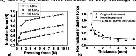
**Figure 2.** Indenter force of the novel instrument (elastic isotropic FE model) as a function of the pressing force for three material stiffness (5, 10 and 20 MPa) (a). The experimentally determined normalized indenter force for the original instrument as well as both experimentally and numerically (elastic isotropic FE model) determined indenter forces for the novel instrument as a function of the elastomer thickness (b).
