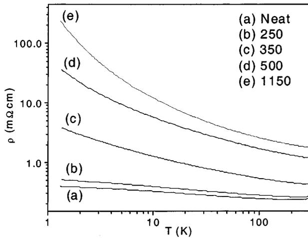
FIG. 6. Effect of vacuum annealing on  $\rho(T)$  for HPR93B; note log-log scale.  $\rho$  increases as the bisulfate  $\rho$  dopants are removed, especially at very low  $T$  (factor  $\sim 500$  at 1.3 K).
