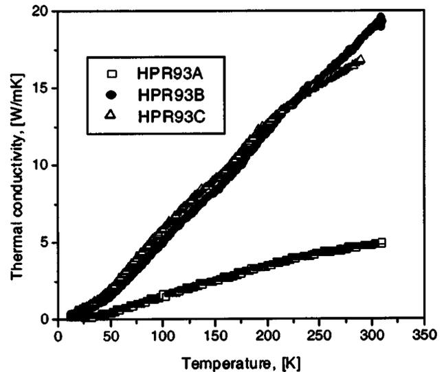
FIG. 8. Thermal conductivity  $\kappa$  vs temperature of the three fibers, measured using the comparator method.
