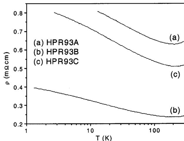
FIG. 5. Four-point resistivity vs temperature for the three neat fibers.  $\rho$  decreases at all  $T$  as alignment improves. Nonmetallic behavior at low  $T$  levels off as  $T \rightarrow 0$  (nondivergent behavior) while metallic behavior is observed above 200 K.
