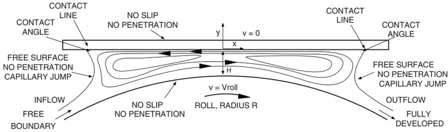
**FIG. 1.** Boundary conditions on the mesh, momentum, and continuity equations in the roll-knife coating flow. At the inflow a free boundary condition is used. At the outflow the flow is fully developed. No-slip and no-penetration condition was applied at the solid boundaries (roll and the coverslip). The position of the contact lines that the free surfaces make with the coverslip was not fixed, but the contact angle was fixed. A capillary force balance was used at the free surfaces.
