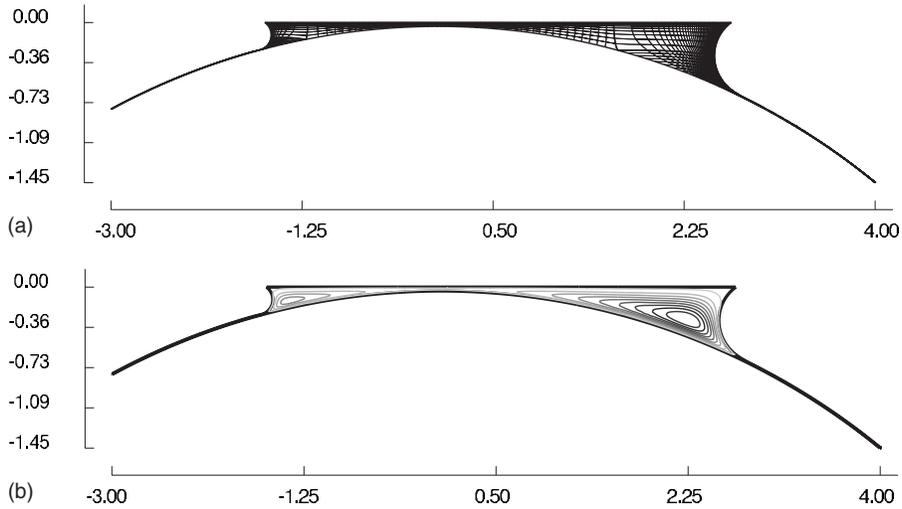
**FIG. 2.** (a) Finite element mesh solution (2600 elements, 50 844 degrees of freedom) of the roll-knife coating flowcell. The dimensions are in mm. The radius of the roll is  $R=6.35$  mm and the gap is  $H=35.3$   $\mu\text{m}$ . The capillary number of the flow was  $\text{Ca}=0.0011$ . The results correspond to the low capillary number experiments E4 and E8 (Duggal and Pasquali, 2004). (b) Streamlines showing the large recirculation below the coverslip.
