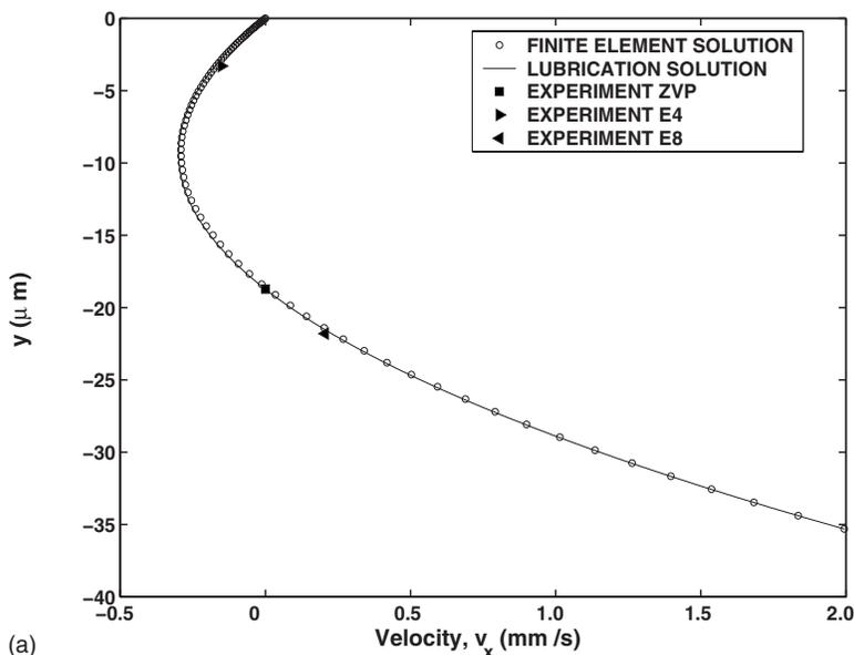
**FIG. 3.** Comparison of the velocity profile at minimum gap ( $x=0$ ) computed by finite elements  $\circ$  and that computed by lubrication approximation (solid line). The experimentally measured velocities at the various image planes (zero velocity plane ZVP, E4, and E8) are also plotted.
