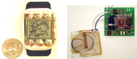
Figure 1. CacheWatch and its PCB with a coin-size battery
