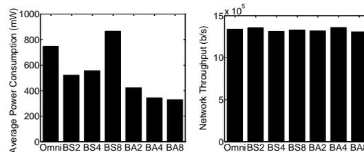
Figure 2. Client power consumption and network throughput of BeamAdapt, beamsteering and omni directional transmission
