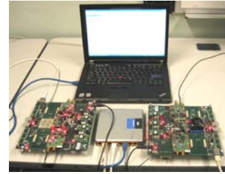
Figure 6. One laptop and two WARP nodes in the prototype
