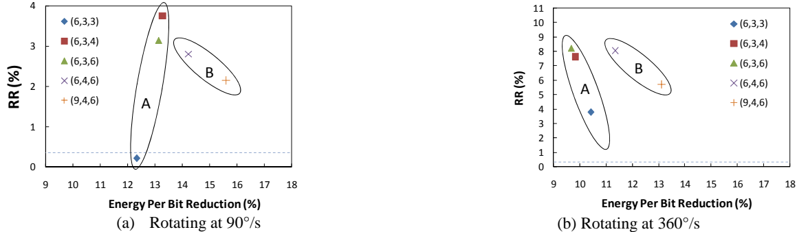
Figure 12: Tradeoffs between retransmission rate (RR) and energy per bit reduction by various RF configurations for VoIP. Dashed line shows the retransmission rate of a conventional omni antenna-based system
