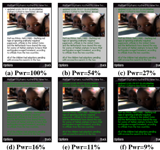
Figure 1: Chameleon first transforms the original GUI (a) to a new GUI (f) with minimal power consumption; and then automatically generates a series of color schemes (b)-(e) with graduate transitions in visual perception. The display power consumption of each GUIs (a)-(f) decreases from 100% to 9%.
