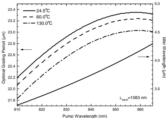
**Fig. 2.** Computed tuning characteristic of a quasi-phase-matched PPLN crystal at a fixed signal wavelength of 1083 nm. Shown is the optimal grating period at three temperatures of 24.5, 60, and 130  $^{\circ}\text{C}$  and the generated idler wavelength as a function of the pump wavelength
