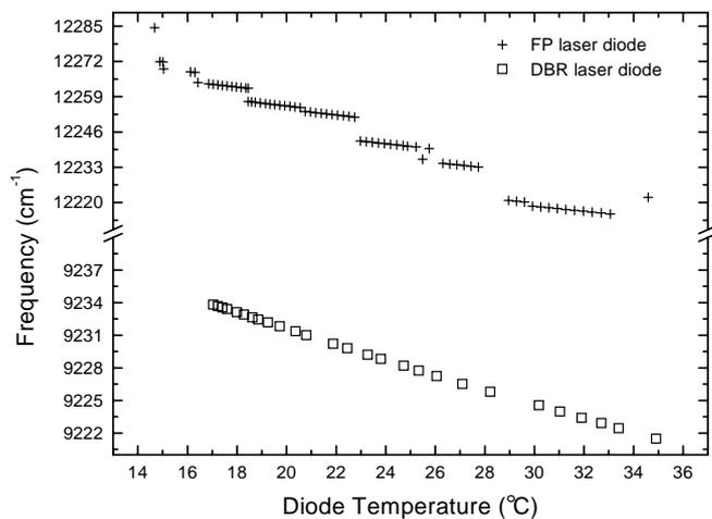
**Fig. 3.** Diode laser wavelength tuning characteristics: frequency vs. diode laser temperature
