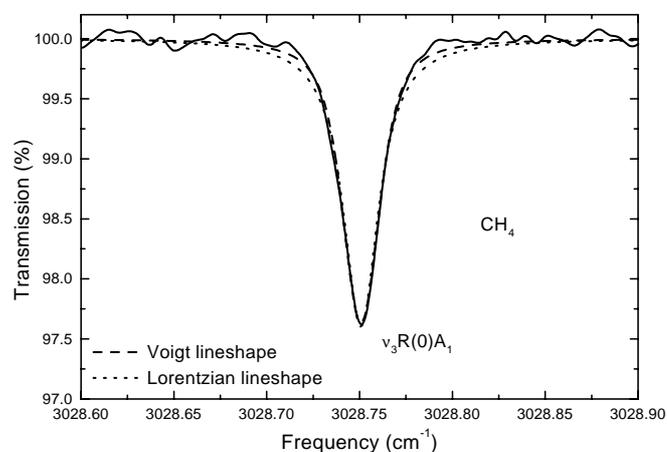
**Fig. 5.** Interference-free absorption line of  $\text{CH}_4$  at  $3028.751 \text{ cm}^{-1}$  obtained with a calibrated gas sample [NOAA, 1998] at a pressure of 100 Torr
