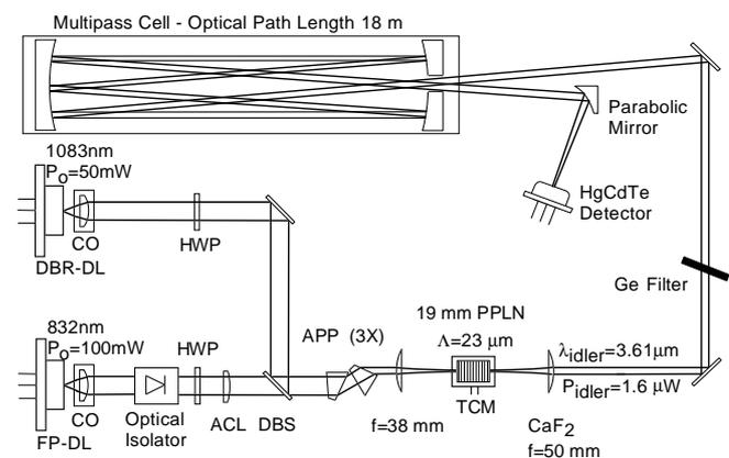
**Fig. 1.** Schematic of the diode-laser-based mid-infrared DFG sensor. CO, collimation optic; HWP, half wave plate; ACL, astigmatism correction lens; DBS, dichroic beam splitter; APP, anamorphic prism pair; TCM, temperature-controlled PPLN crystal mount
