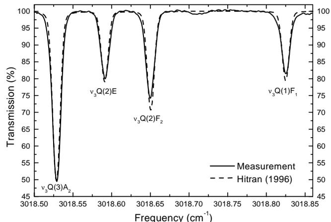
**Fig. 4.**  $\text{CH}_4$  spectrum in the Q branch at  $3.31 \mu\text{m}$ . A small volume of methane was added to the gas-handling unit. The multi-pass cell was then sealed for spectral measurements at a pressure of 10 Torr
