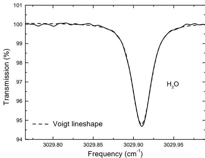
**Fig. 6.** H<sub>2</sub>O absorption line at 3029.91 cm<sup>-1</sup> measured in ambient air at 100 Torr
