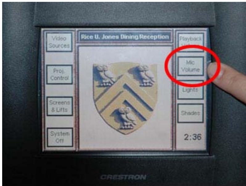
\*Adjust the volume to a comfortable level by pushing the up or down arrow on the area marked MICROPHONE VOLUME.
