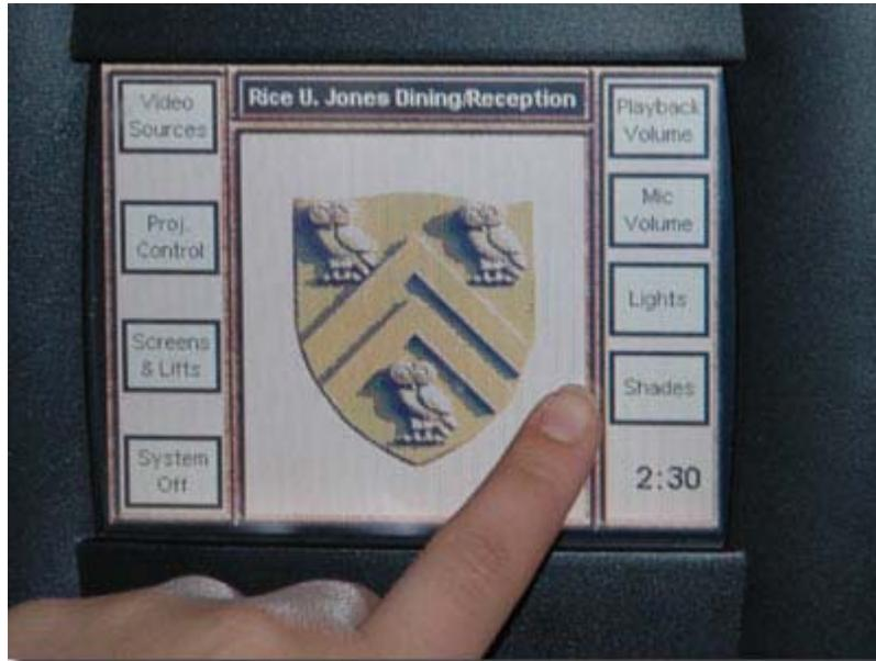
\*A window will open up with up and down arrows allowing you to raise or lower the shades.
