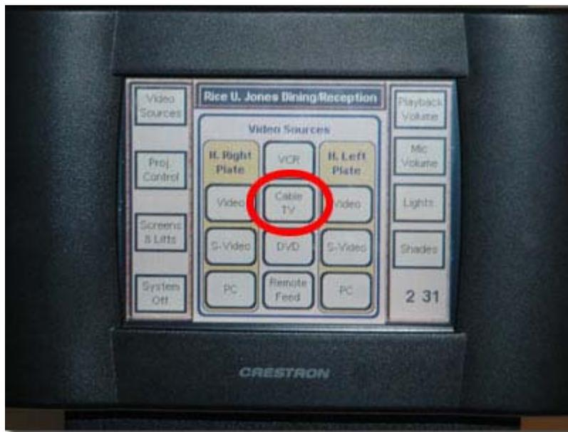
\*Press the CABLE TV button. When you do this – you will be asked whether you want the image on both projectors or just one. Then Cable TV control window will appear. Also, the Screen(s) will lower, LCD projector(s) will power up and Cable TV will route to the projector(s).
