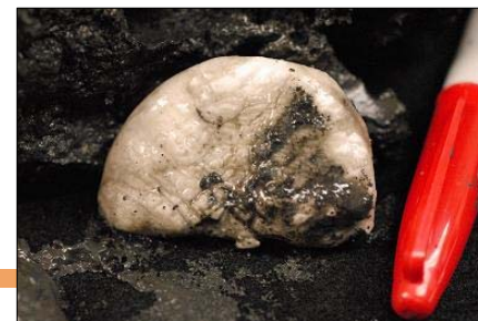
Massive hydrate sample from offshore India – NGHP Expedition 01
