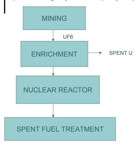
Diffusion, Centrifuges, Thermal, Becker Nozzle, etc.
