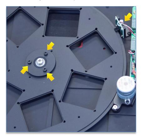
6: Now lift the carousel off the hub and away from the sensor, taking care not to damage the optical sensor.
