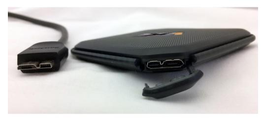
Figure 280: Plug this end of the USB cable on the left into the SSD drive's input port.
