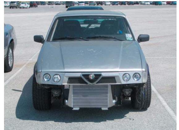
The high-performance radiator in place before bumper installation
