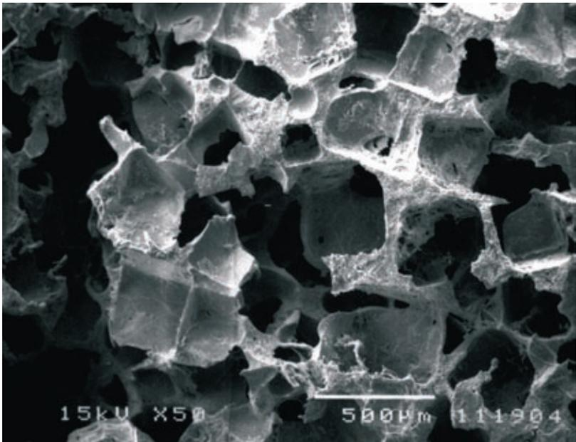
Figure 1: Porous, biodegradable scaffolds obtained by photo-cross-linking a polymer around a pore-forming chemical (sodium chloride).
