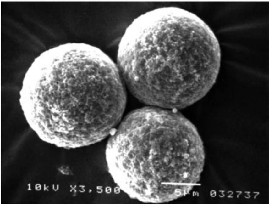
Figure 3: Biodegradable polymer microparticles, commonly used in drug delivery strategies, display rough surface characteristics after 14 days of degradation.
