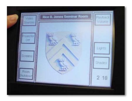
\*Locate and press the VCR button – in the center column of buttons. When you do this – the Screen will lower, LCD projector will power up and the VCR will route to the projector.
