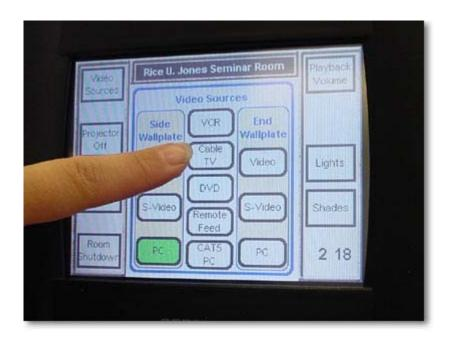
\*Press the CABLE TV button. The Cable TV control window will appear. Also, the Screen will lower, LCD projector will power up and Cable TV will route to the projector.
