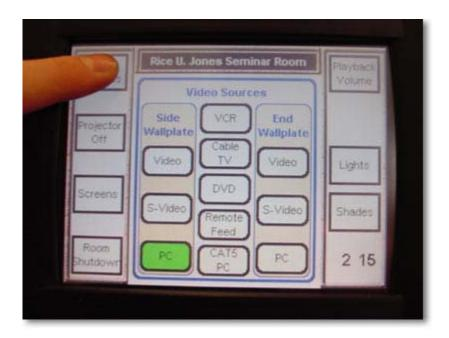
\*Should you want to interrupt the display of your source, simply touch the "Projector Off" button. To resume the display, select your source again and press the "Send to Projector" button.
