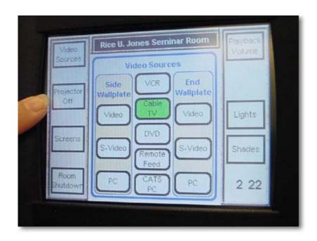
\*When this button is pressed, it puts the LCD Projector in mute for 15 minutes. If the projector is not reactivated before this time is up, the projector will fully power down.
