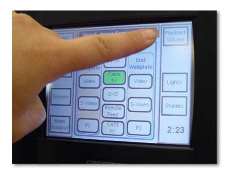
\*Adjust the volume to a comfortable level by pushing the up or down arrow on the area marked PLAYBACK VOLUME.
