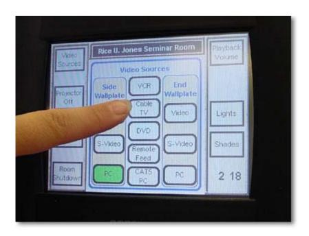
\*Locate and press the DVD button – in the center column of buttons. When you do this – the Screen will lower, LCD projector will power up and the DVD will route to the projector.
