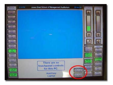
\*When this button is pressed, it puts the LCD Projectors in mute for 15 minutes. If the projector is not reactivated before this time is up, the projectors will fully power down.
