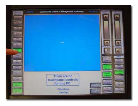
\*You can touch the center of the touch screen and view an enlarged preview area. When you want to go back to the touch panel controls, touch the center of the screen again.
