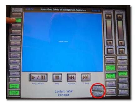
\*Should you want to interrupt the display of your source, simply touch the LEFT PROJECTOR OFF and RIGHT PROJECTOR OFF buttons. To resume the display, select your source again and press the SEND TO LEFT PROJECTOR" and SEND TO RIGHT PROJECTOR buttons.
