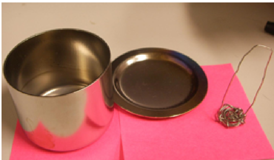
Figure B.1 : Cr crucible and basket are used for pit-etching with KOH.
